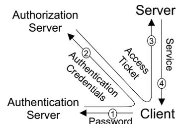
Fig. 1. Our access model: We separate the access control process into three steps: authentication, authorization and access verification. Each step may be handled by a separate server on the network.
