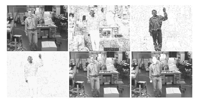
Figure 2: Different stages of the detection process. (a) sample camera image (b) potential skin color pixels (c) foreground pixels (d) foreground skin color pixels (e) cluster bounding boxes (f) centroids and first moments of clusters.
